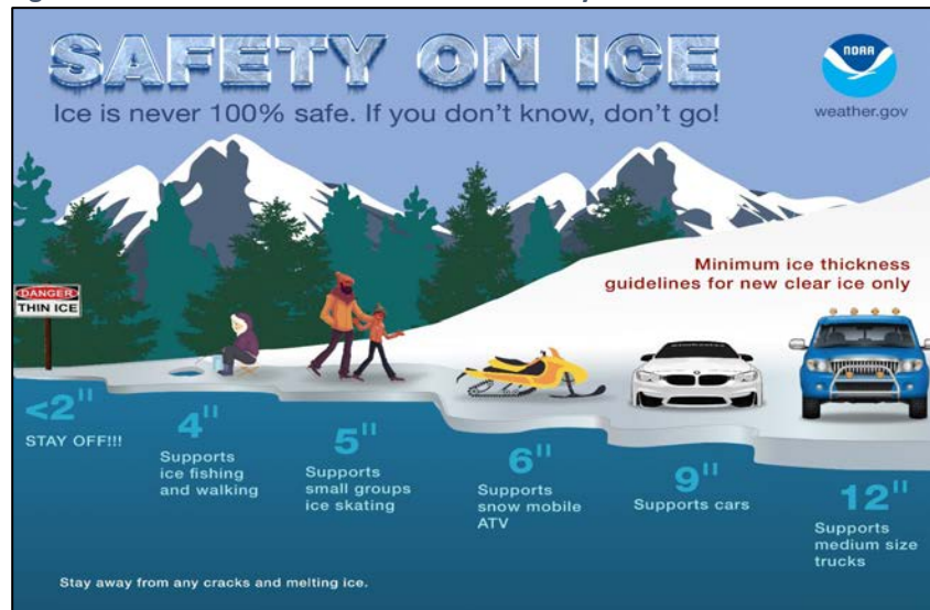
Figure 4.5-42: Minimum Ice Thickness for Safety
