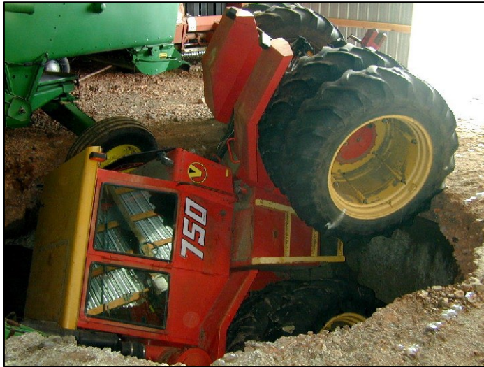
Figure 4.12-32: Tractor in an Abandoned Mine Land Sinkhole
